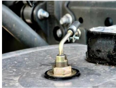
A type fuel suction pipe
